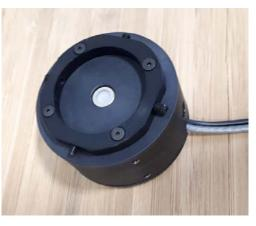
The spectral range is limited by high density polyethylene window.
